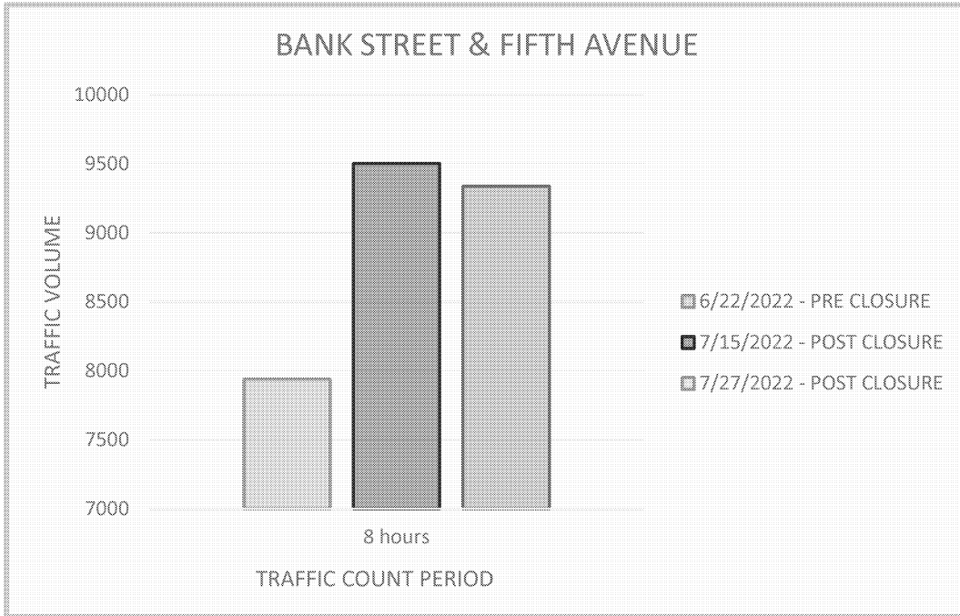
Figure 2 - Total Traffic Volume (8hr) at the intersection of Bank Street & Fifth Avenue
